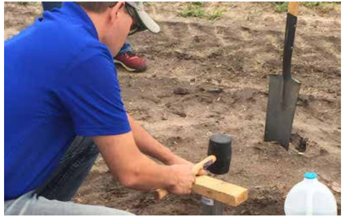
Figure 2. One of the methods for soil health sampling is to use a steel bulk density ring that is pounded into the ground with a block of wood and mallet, then the ring and soil sample is removed with a shovel. This method preserves the inherent structure of the soil, allowing bulk density to be measured, and also provides a good quality sample for other soil health tests. (Credit: R. Koelsch)
